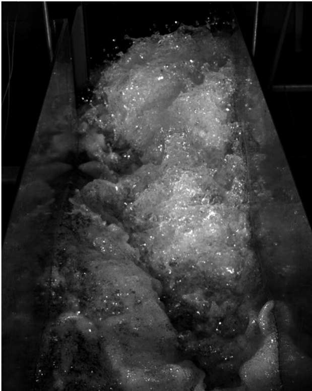
Figure 4. Confluence flow is highly turbulent, here recorded with secondary camera from position shown in Fig. 2.
