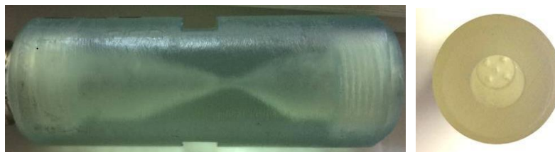
Figure 1: Pictures of the Venturi tube and orifice plate devices used for the experiments.
