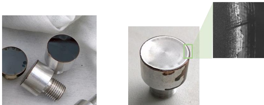
Figure 1: Specimens with coking layers before and after cavitation exposure.
